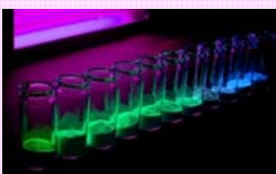
(\text{Sr}_{1-x}\text{Ca}_x)\text{O} \cdot n\text{Al}_2\text{O}_3:\text{Eu}^{2+},\text{Dy}^{3+} samples excited by UV radiation (366 nm)
