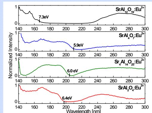
Excitation spectra of  $x\text{SrO}-y\text{Al}_2\text{O}_3$  doped with  $\text{Eu}^{2+}$
