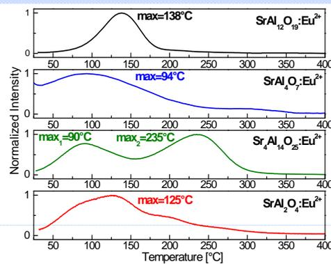
TL spectra of  $x\text{SrO}-y\text{Al}_2\text{O}_3$  doped with  $\text{Eu}^{2+}$
