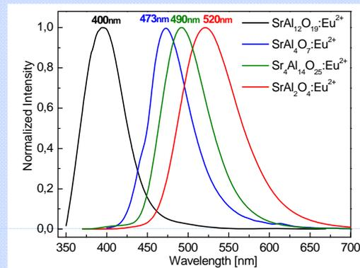
Emission spectra of  $x\text{SrO}-y\text{Al}_2\text{O}_3$  doped with  $\text{Eu}^{2+}$
