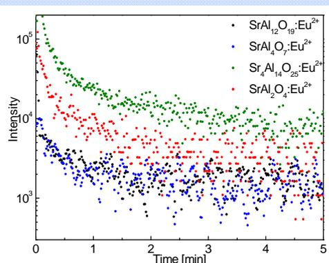
Decay curves of  $x\text{SrO}-y\text{Al}_2\text{O}_3$  doped with  $\text{Eu}^{2+}$
