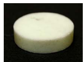
Fig. 8 Example of a typical translucent KY 3 F 10 :Pr 3+ ceramic
