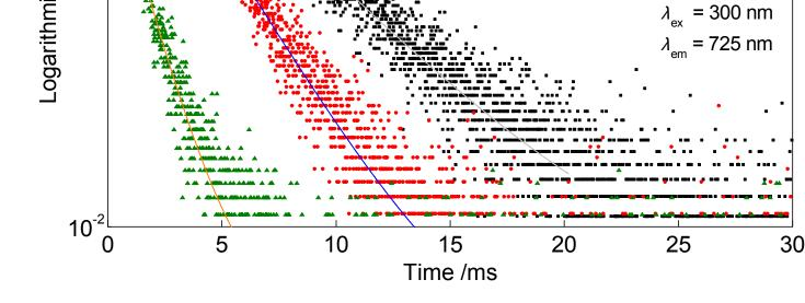
Fluorescence lifetimes of Mn<sup>2+</sup> start to decrease at lower temperature compared to those of Ce<sup>3+</sup> indicating that thermal quenching is mainly caused by Mn<sup>2+</sup>.
