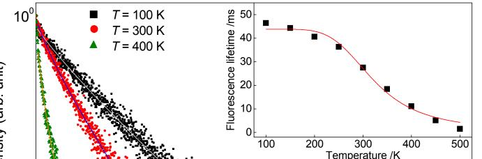
Fluorescence lifetimes of Ce<sup>3+</sup> remain constant up to about 350 K reflecting the good temperature stability of the internal quantum efficiency of Ce<sup>3+</sup>.
