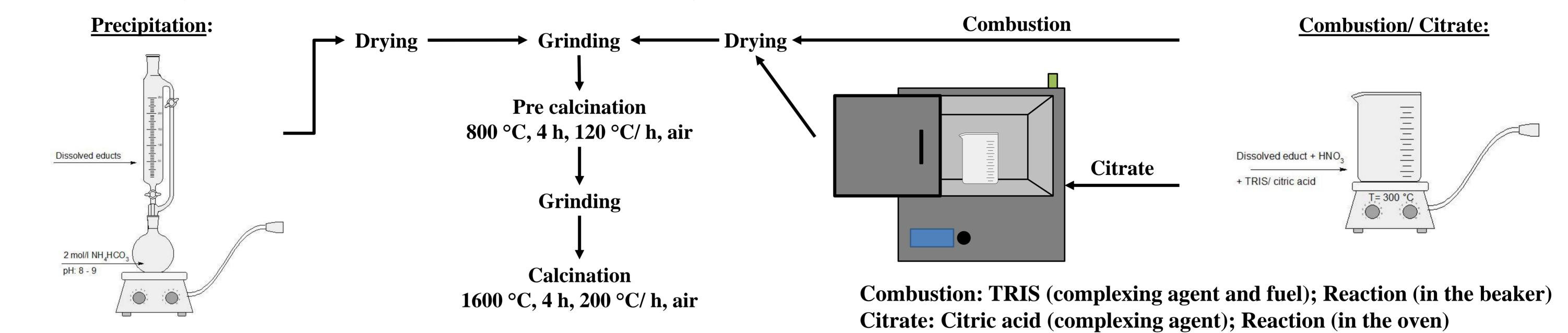
The educts precipitate as hydroxy carbonates
