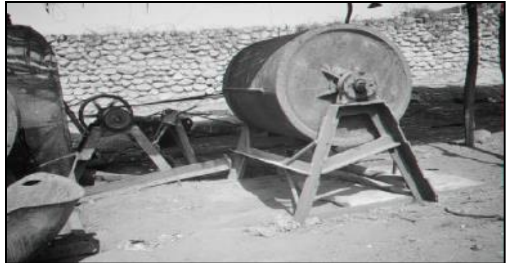
A ball mill being used as part of a gold mining operation in Peru
