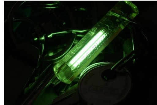
Tritium filled tube coated with \text{Zn}_2\text{SiO}_4:\text{Mn}^{2+}
