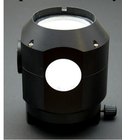
\text{BaMgAl}_{10}\text{O}_{17}:\text{Eu} coated integration sphere under daylight or upon VUV exc.
