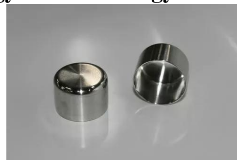
Iridium crucibles ( T_m = 2465^\circ \text{C} )
