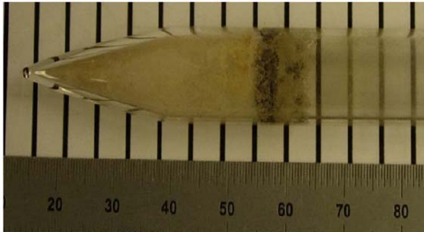
A 1 cm in diameter \text{Ba}_2\text{CsI}_5:\text{Eu}^{2+} shown as-grown in a sealed quartz ampoule.
