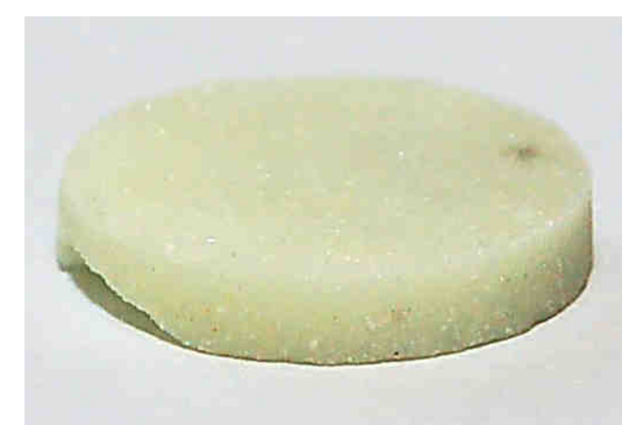
Fig. 6 Example of a typical translucent LiYF 4 :Pr 3+ ceramic
