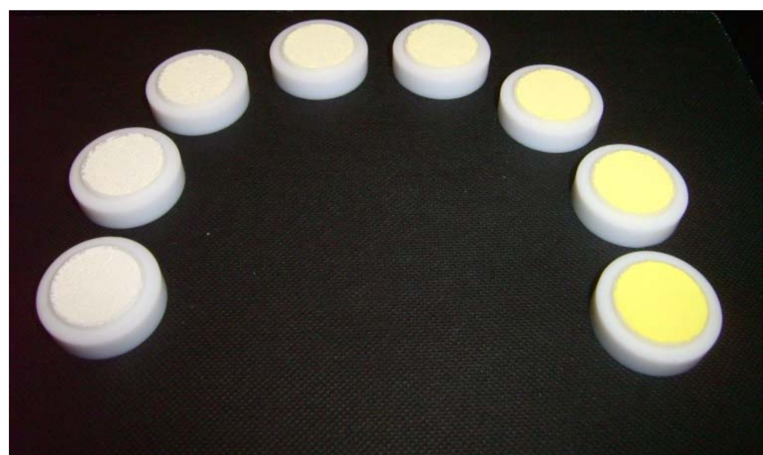
Fig. 4: Sample holder with YAG:Ce (U819)/ BaSO_4 - concentration series. Increasing YAG:Ce content 1 % (left, bottom), 2 %, 5 %, 10 %, 20 %, 40 %, 60 %, 80 % (right, bottom)
