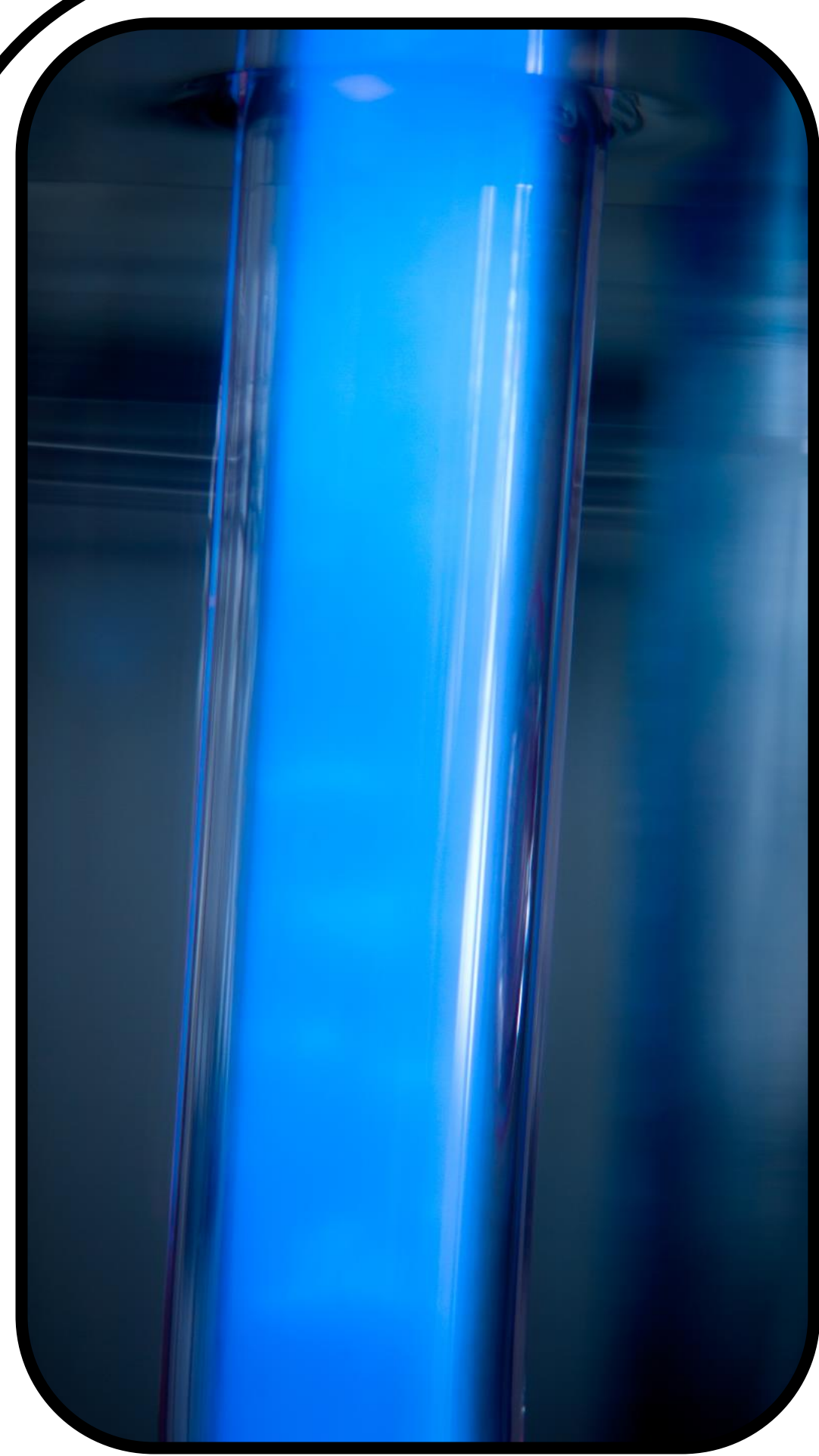
Fig. 2 Coaxial Xe-DBD Lamp operated in water.
