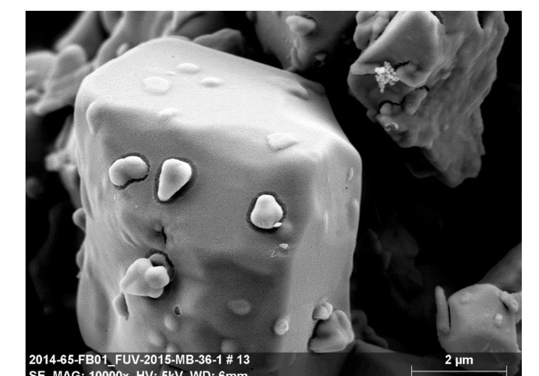
Fig. 7 SEM image of Al 2 O 3 coated YPO 4 :Bi particle
