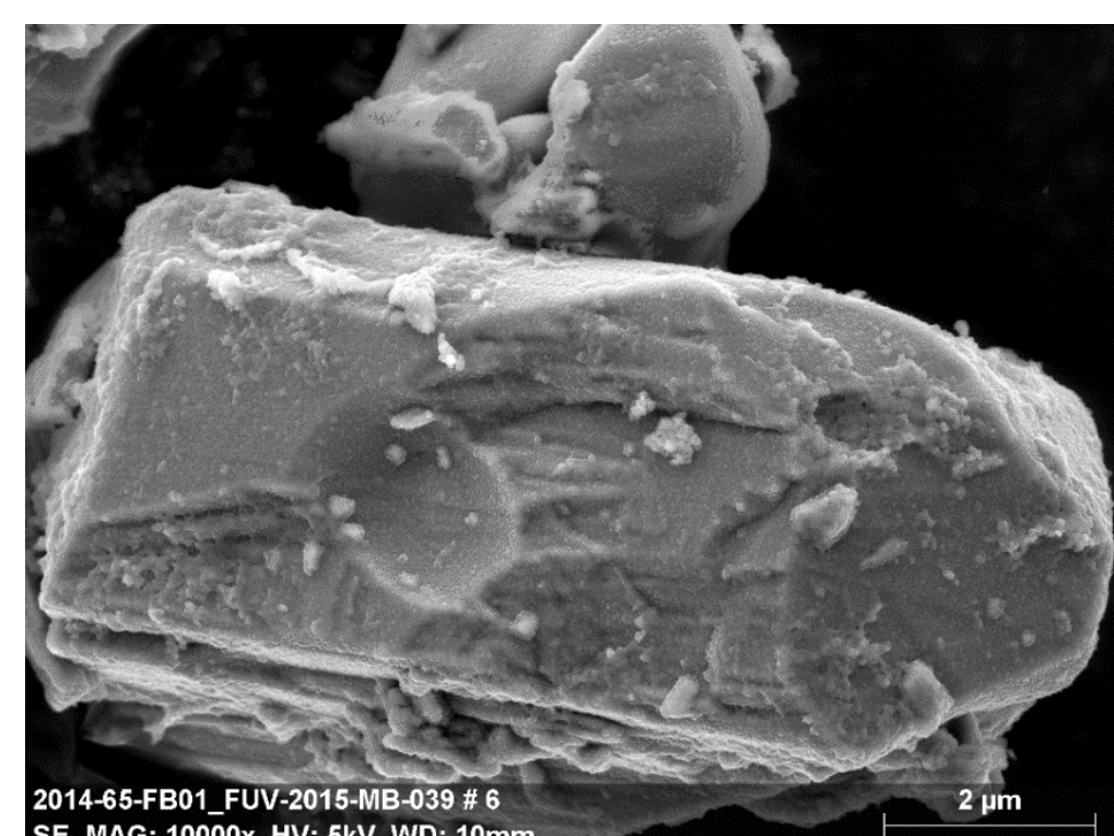
Fig. 3 SEM image of Al 2 O 3 coated YPO 4 :Bi particle
