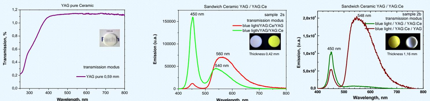
Transmitted emission spectra of the sandwich YAG/YAG:Ce ceramics measured under irradiation with the blue light - 450 nm.
