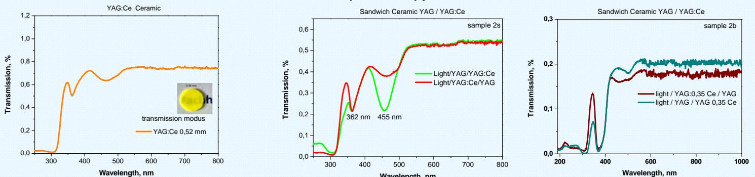
Transmission spectra of the sandwich YAG/YAG:Ce ceramics.
