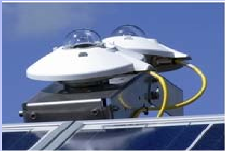
Horizontal and tilted pyranometer (left, courtesy skytron energy ) Pyranometer CMP11 (right, courtesy: Kipp & Zonen )
