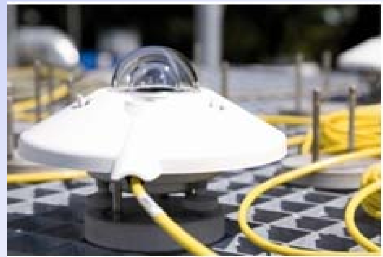
Horizontal and tilted pyranometer (left, courtesy skytron energy ) Pyranometer CMP11 (right, courtesy: Kipp & Zonen )
