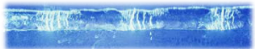
PT using fluorescent penetrant under black light
