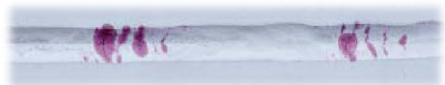
PT using visible penetrant and developer
