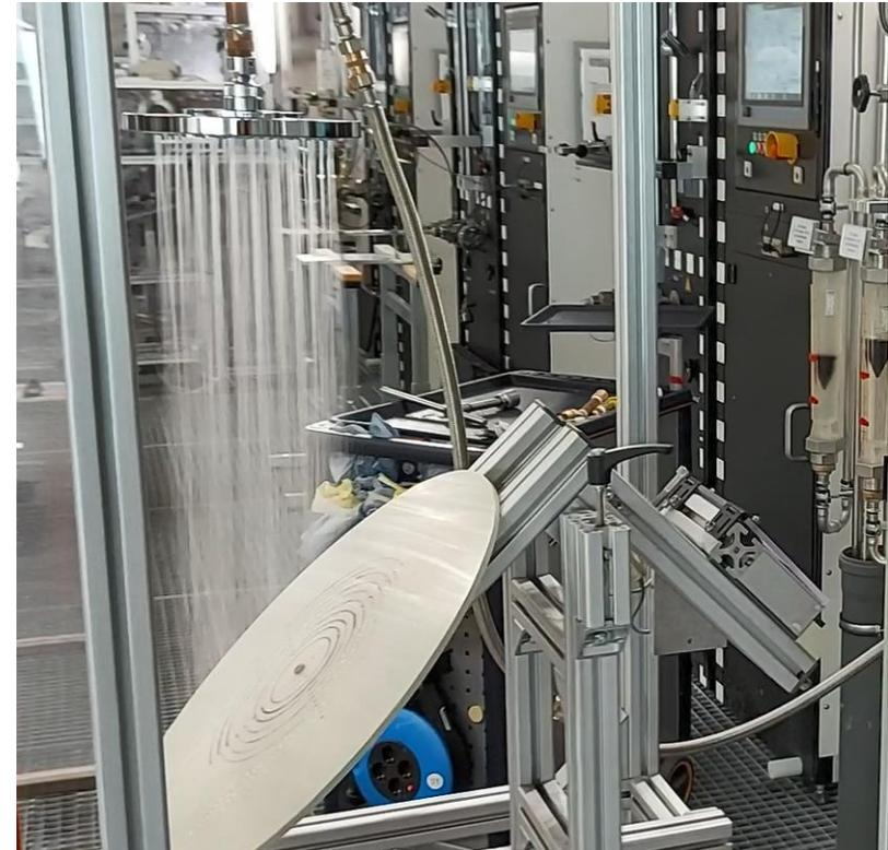
Strahlkraft (WaterSense Spray Force Test)
