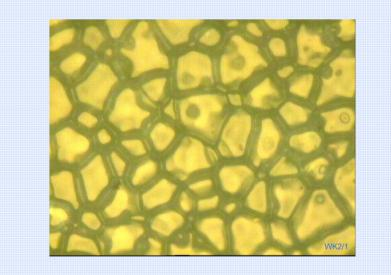
**Microstructure and Image of** ceramics YAG:Gd,Pr (sintering 1650 and 1700 °C for 12h)
