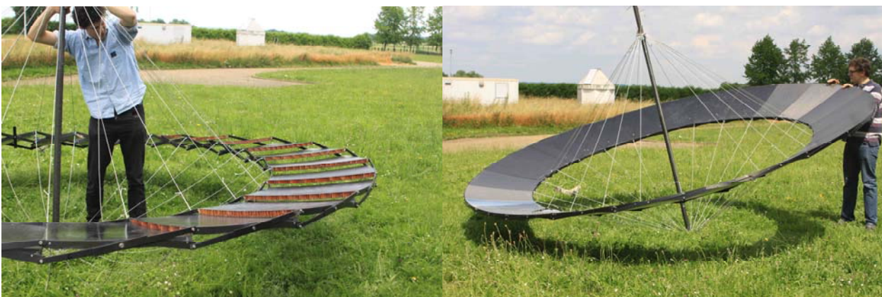
Figure 5. The scissors are made of pre-impregnated UD carbon epoxy. We learned that a synchronization system is needed between the inner and outer scissors to help the pack of segments extend on a predictable trajectory. In the next model the toggling scissors will be tubular. The inner and outer scissors will be built as a single piece in shape of C.
