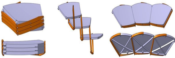
Fig. 6. Deployment of subset of segments of TALC to be tested in cryogenic conditions
